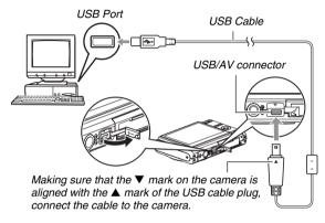
When connecting the bundled USB cable to the camera's USB/AV port, insert the plug into the port until you feel it click securely into place. Failure to insert the plug fully can result in poor communication or malfunction of the connected components.  Some metal of the plug is visible even when the plug is inserted correctly.
